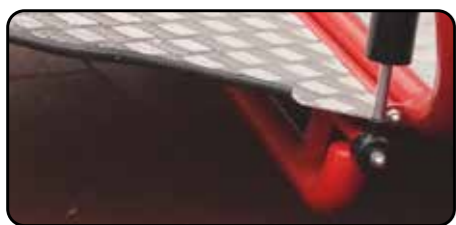
Skid-shaped gondola's stabilizer making easier entry for wheelchair
